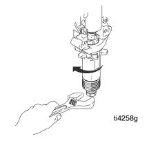
12. Remove pin and piston rod from cylinder.
