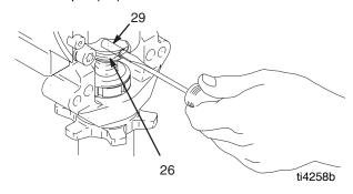
5. Disassemble intake valve. Clean and inspect. O-ring (227) may require a pick for removal.
