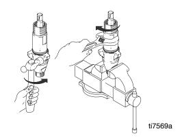
13. Torque packing nut (202) as follows:
