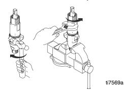
3. Disassemble intake valve. Clean and inspect o-ring (227).
