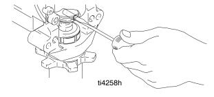
13. Soak all leather packings in SAE 30W oil for 1 hour minimum prior to assembly. Stack male gland (204). Alternately stack UHMWPE (203) and leather (223) packings (note orientation). Install female gland (224). Install seal (201) and packing nut (202) and o-ring (228).
