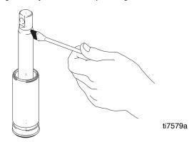
9. Grease o-rings (221) and place on sleeve. Slide sleeve/piston rod assembly into bottom of cylinder. Replace o-ring (207) if desired.
