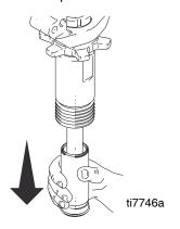
Invert piston rod and sleeve and pound on hard surface until piston rod comes out of sleeve.
