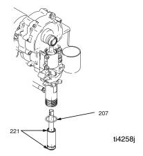
21. Torque seal and packing nut (202) to the following:
