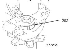
9. Invert piston rod and insert into cylinder to force out throat packings.
