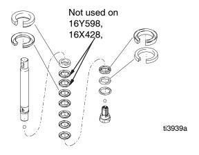
15. Soak all leather packings in SAE 30W oil for one hour minimum prior to assembly. Stack male gland (219) on piston rod. Alternately stack UHMWPE (208)and leather (218) packings (note orientation) on piston rod. Install female gland (217). Install piston wiper (216) and backup washer (229) (note orientation) on piston valve (210). The special sealing patch on piston valve threads is good for four repackings. Use thread sealant on piston valve threads after four repackings.
