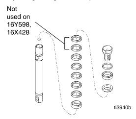
8. Remove throat packings and glands from cylinder. Discard throat packings and glands.
