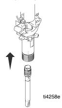
Insert piston rod into cylinder with pin hole up and piston valve down. Insert pin into piston rod and crank shaft.
