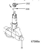
2. Unscrew intake valve from cylinder.
