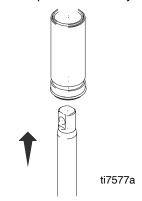
8. Grease top inch or two of piston rod that will go through the cylinder throat packings.
