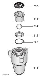
25. Install intake valve on cylinder. Torque as follows:
